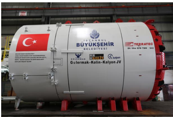
TERRATEC Ø6.56m EPB TBM for Istanbul Metro
