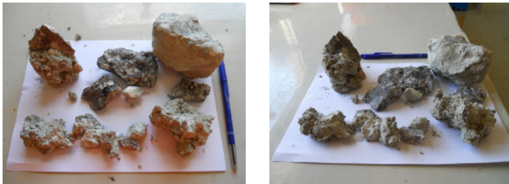
Figure 6. Ground excavated in the WS5 at the TBM depth
