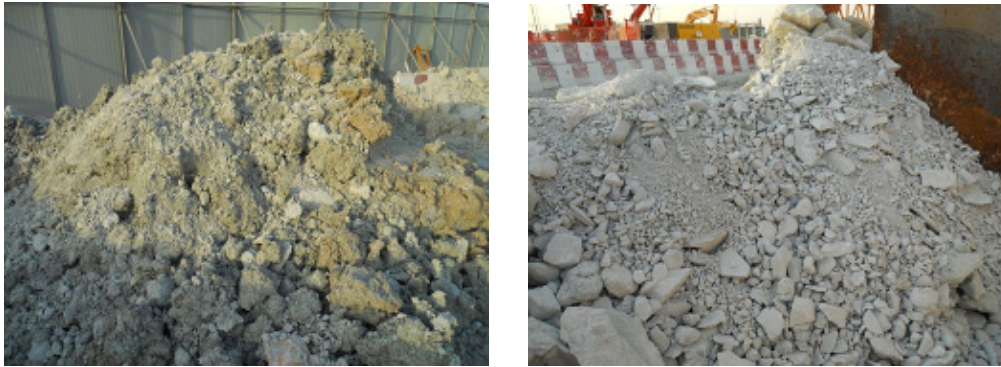
Figure 6. Ground excavated in the WS5 at the TBM depth
