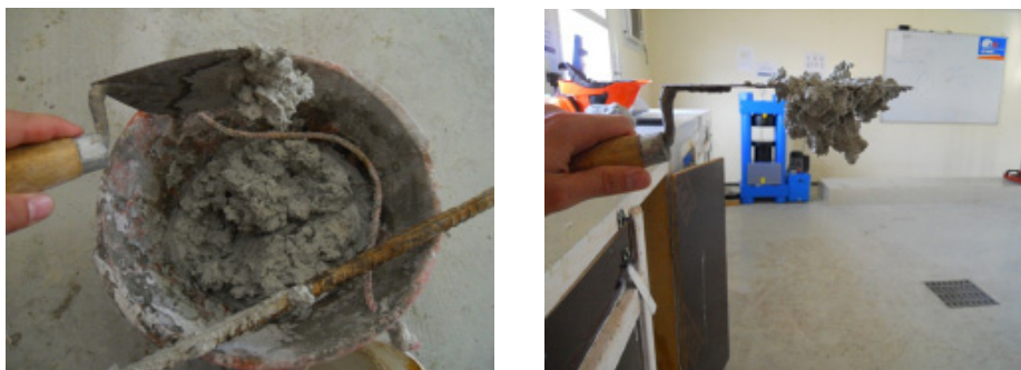
Figure 8. Addition of pure water to the ground and thixotropic properties of the wetted material
