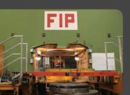
FIP INDUSTRIALE productive headquarters are in Padua, close to Venice in Italy. They are equipped with the most modern laboratory for static and dynamic testing of materials and devices, including one of the largest presses in the world, having 80000 kN of vertical load and 7500 kN of horizontal load. The equipment and competence of the laboratory permit the company to satisfy the most complex experimental and testing requirements, also for every kind of tunnel condition.
